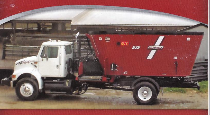
Models 625, 745 and 865 truck, trailer or stationary with twin augers
